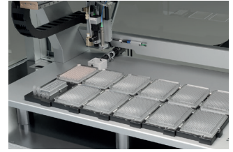
High speed XYZ axes, top speed: 1000 mm/s
