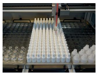
One of four possible trays loaded in this example with 162 bottles of 16 mL filling volume capacity.
