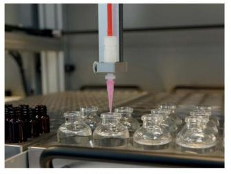
Bottle by bottle will be filled with the same volume of the supplied solution (here: 30 mL).
